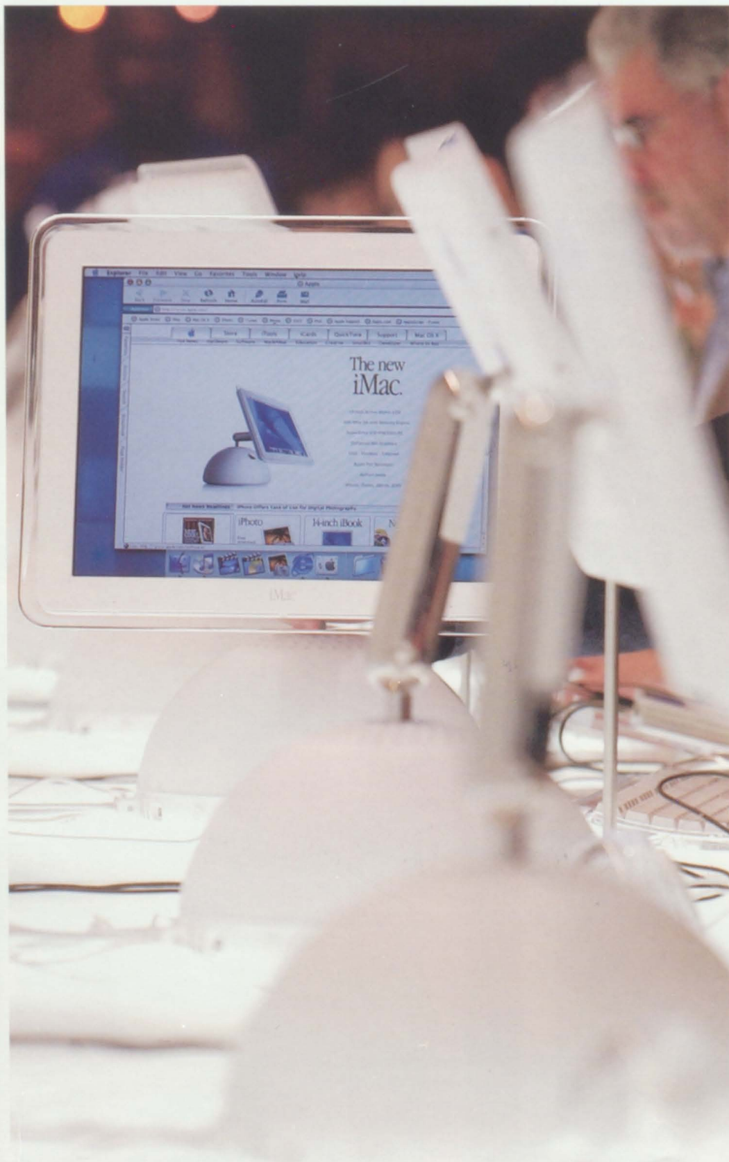
A new top-of-the-line iMac is introduced by Apple Computer. The redesigned computer has a floating 15-inch LCD flat screen, allowing users one-touch adjustment, a 700 MHz or 800 MHz PowerPC G4 processor, and the SuperDrive for playing and burning CDs and DVDs.
